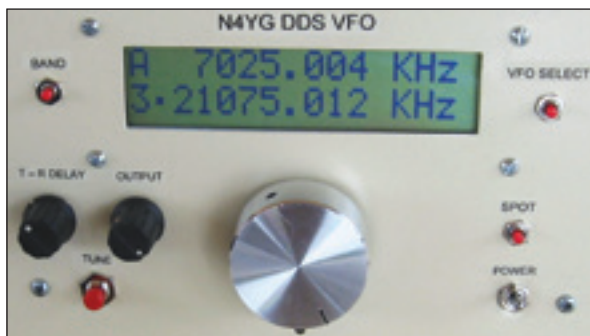
Figure 1 — The stand-alone DDS VFO, suitable for frequency control of '50s transmitters such as Johnson Ranger, Adventurer, Navigator or Viking; Heathkit AT-1, DX-20, 35, 40, 60 or 100.
