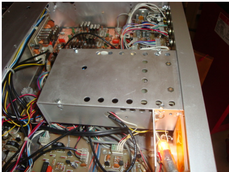
Figure 7. LED Readout Enclosure – Top View
