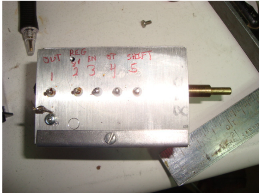
Figure 2. PTO ready to go on the shelf (Labeling is useful for any future use.)
