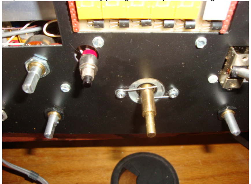
Figure 3. PTO Shaft and Grounding Springs
